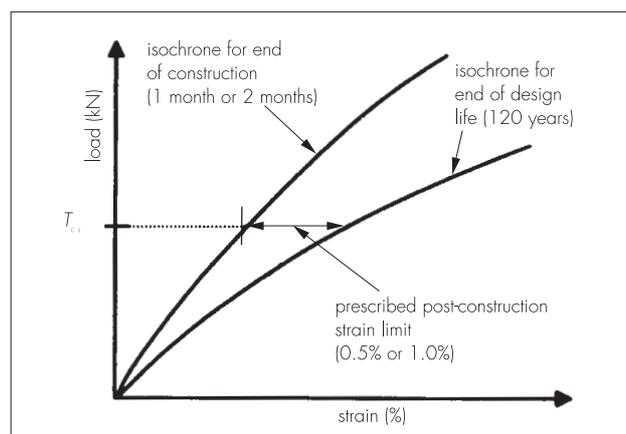
6.4 Isochronous curves based on long-term creep strain tests have been derived (see Figure 4). From these curves values for  $T_{CS}$  have been calculated and it has been found that creep rupture, as opposed to creep strain, governs the long-term performance of the geogrid.  $T_{CS}$  values, therefore, can be taken as the corresponding  $T_{CR}$  value.
