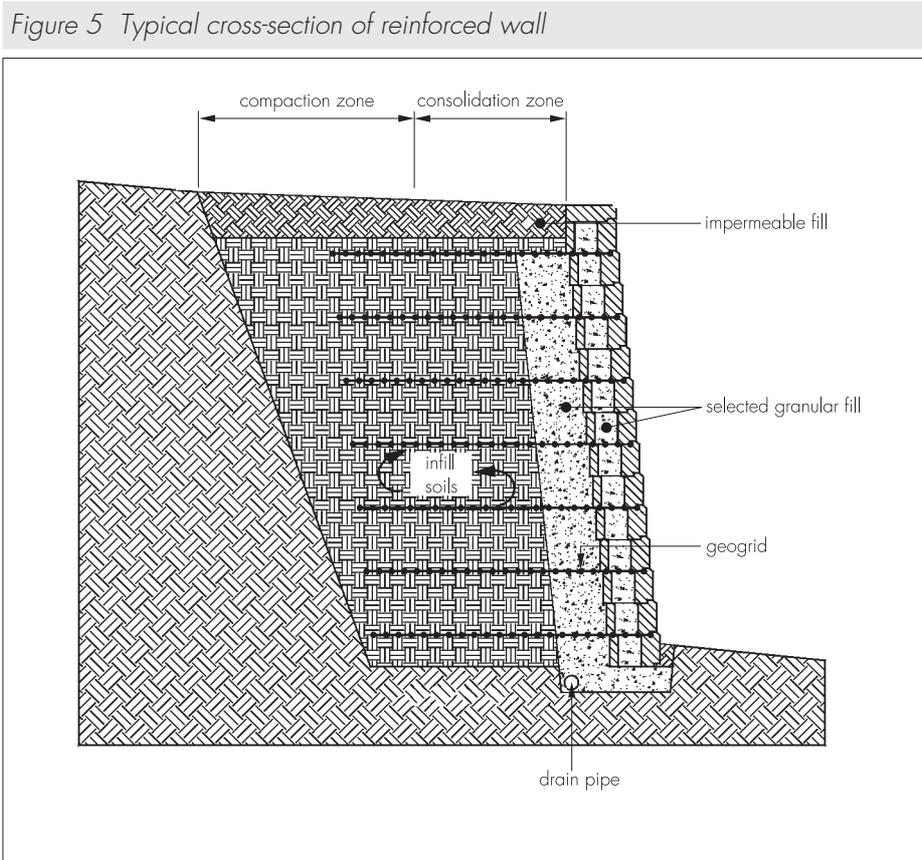
10.2 The blocks are laid on a levelling pad composed of either well-graded, good compactable material ranging in diameter from 6 mm to 38 mm or a suitable concrete foundation laid to the correct level for the first course of facing units. The first course of the wall units are laid and checked for level and alignment.
